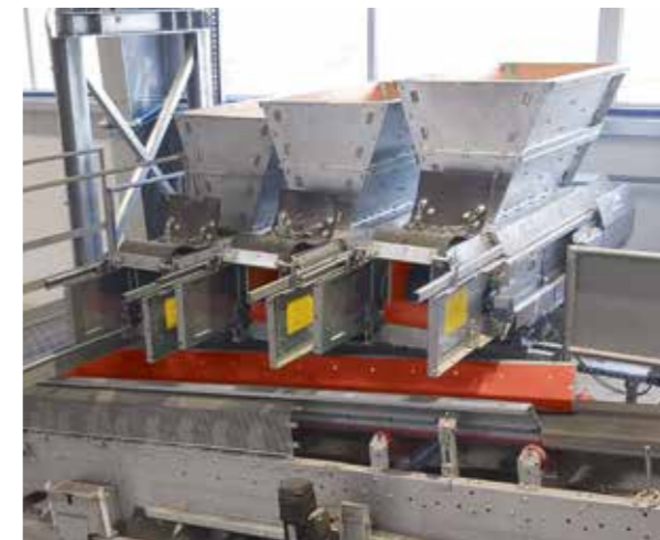
Color-Mix shuttle belt system
